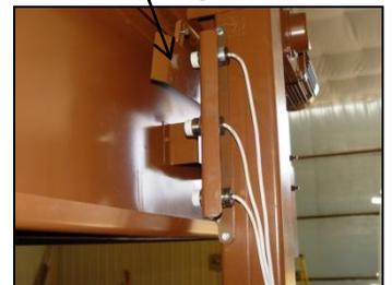
**Step 11:** The Proximity Sensor Plate can be adjusted for the length of travel of the shelf conveyor to match the size of your bins. The Lower Proximity Sensor Plate, on the rear of the shelf (Fig. 8), is set approximately 18 inches from the rear of the shelf conveyor. The Upper Proximity Sensor Plate (Fig. 9) is approximately 30 inches from the front of the shelf conveyor. The middle Proximity Sensor Plate, which activates the home position, is factory preset.
