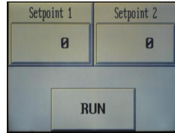
**Step 9:** Press MENU to return to the menu screen (Fig. 3). Then press “Scale”. This will take you to the Scale screen (Fig. 7). On the Scale screen “Setpoint 1” and “Setpoint 2” will appear. Touch “Setpoint 1” to program desired weight for bottom half of box and press enter. Then press “Setpoint 2” to program desired total weight of the tobacco in the box and press enter.
